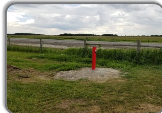
Casing of installed groundwater monitoring well
