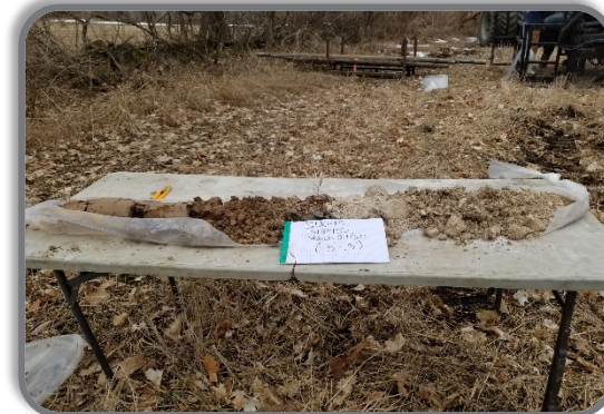
Overburden sampled during exploratory drilling
